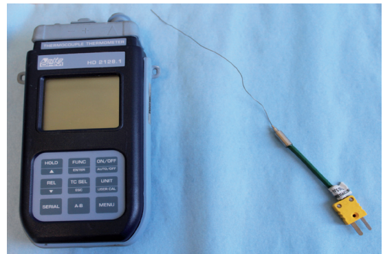
Figure 4.—A two way thermocouple.
