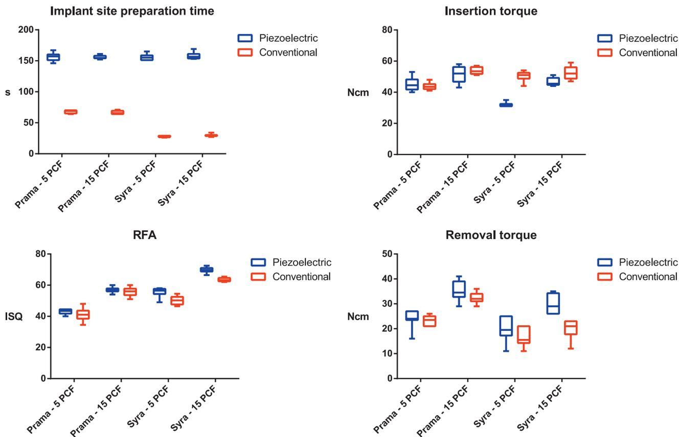
**FIGURE 5.** Box and whiskers plots showing the distribution of the values of the variables of interest of the present study for each considered subgroup (different implant site preparation techniques, implants, and simulated cancellous bone density). ISQ indicates implant stability quotient; PCF, pound per cubic foot; RFA, resonance frequency analysis.
