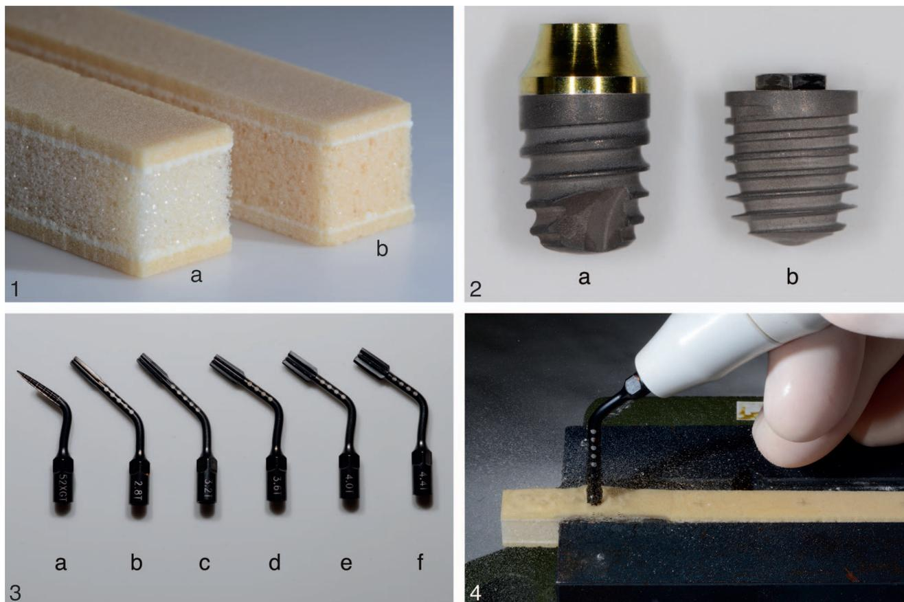
**FIGURES 1–4.** **FIGURE 1.** Bars of custom-made solid rigid polyurethane blocks with different density of simulated cancellous bone. (a) 5 pounds per cubic foot (PCF). (b) 15 PCF. **FIGURE 2.** Tested implants. (a) Prama. (b) Syra. **FIGURE 3.** Sequence of SUS tips for ultrasonic implant site preparation: (a) ES052XGT; (b) ES02.8T; (c) ES03.2T; (d) ES03.6T; (e) ES04.0T; (f) ES04.4T. **FIGURE 4.** Ultrasonic implant site preparation under water irrigation.
