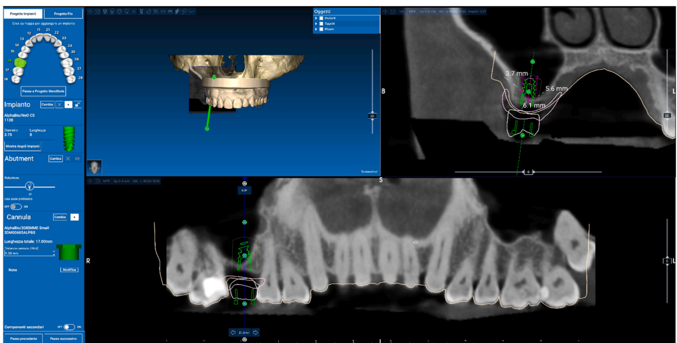
Fig. 1. Illustrative case of virtual planning performed with dedicated software (RealGUIDE, 3DIEMME, Cantù, Italy), which matched and integrated STL and DICOM files from digital dental impression and CBCT scan, respectively.
